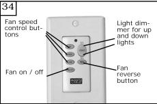
To control fan speed select from High, Medium or low speed buttons. To turn the fan off press the Fan on / off button. To dim upper lights press and hold U/L botton. To dim Lower lights press and hold D/L button. To turn off either up or down light press and quickly release either U/L or D/L button. Press button marked REV to reverse the rotation direction of the fan blades
